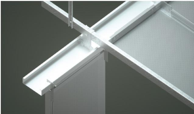
Similar to the flying arm, a hook plate is fixed to the tile edge (supplied loose for on-site fixing by installer). The tile can be completely lifted out of the grid and hooked back over the C-Profile, safely off the ground.
