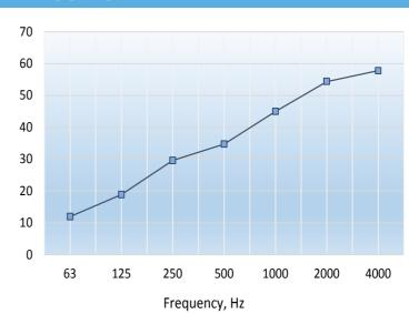
Single figure rating:  $D_{n,c,w}(C;Ctr) = 40$  (-2;-8) dB According to BS EN ISO 717-1: 1997
