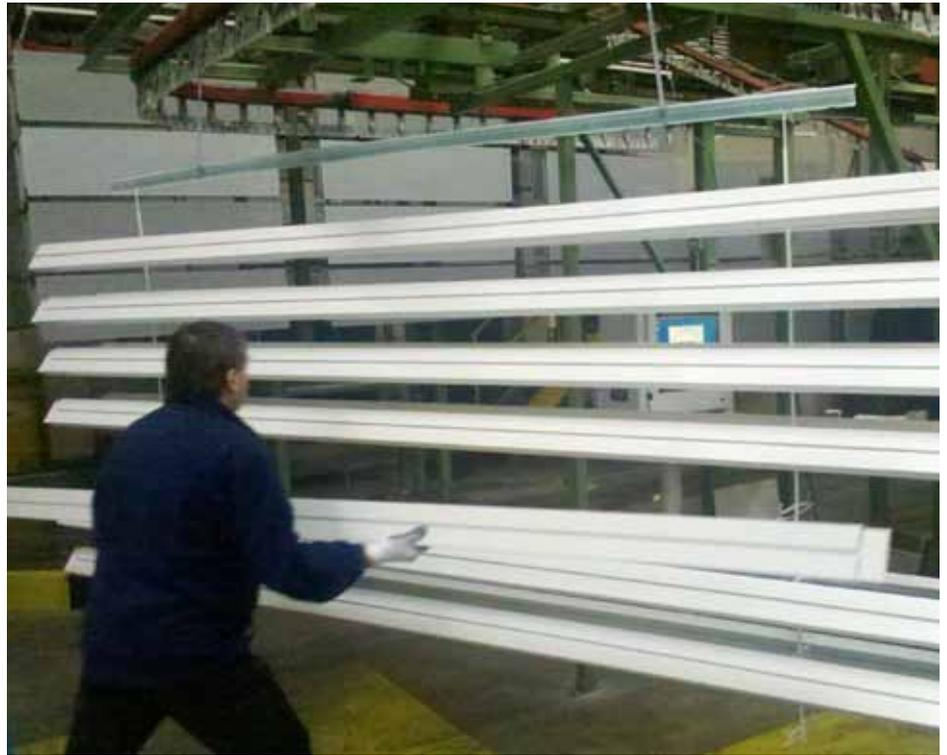
these parts could be painted without additional hand spraying. Not only did this improve the manufacturing cost but improved the lead time immensely as profiles were roll formed at Bridgend and then painted here as well. The photos show the jiggging design needed for consistent paint coverage. This was developed over a 3 week period."
